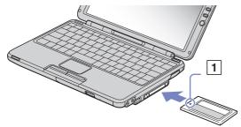
Gently push the card into the slot until the card is fixed into the connector.
